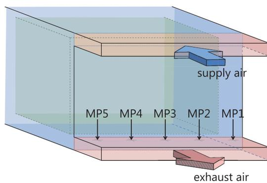
Fig. 2: Measurement positions (MP1...5) at the exhaust (isometric front view)
