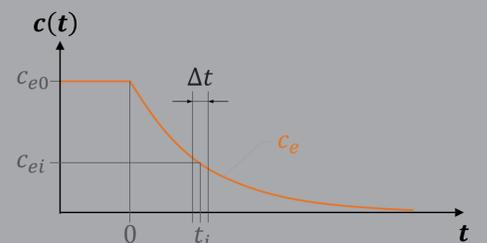
Figure 5: Typical tracer gas concentration decay curve measured in the exhaust air of an ideally mixed flow; according to: Mundt et al (2004)
