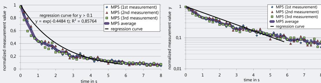
Fig. 4: Linear (left) and single logarithmic (right) diagram of the concentration decay at measurement point MP5 for  $\tau_n = 2,46$  s.
