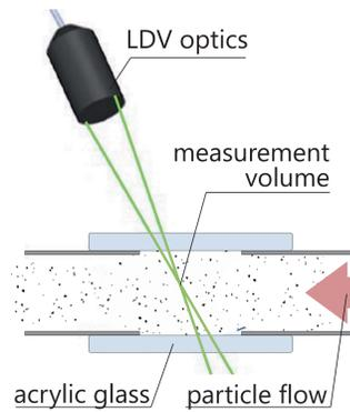
Fig. 3: Measurement position of the LDV focus (cross section)
